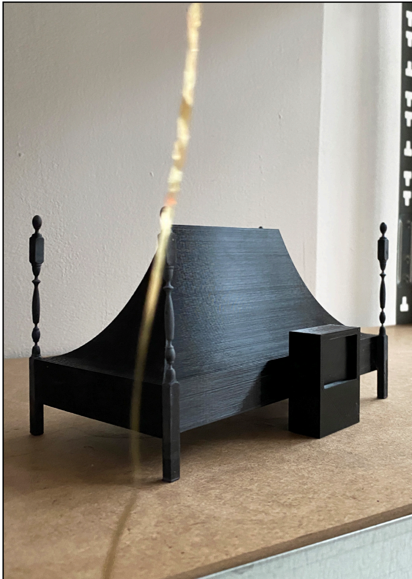
The model of the Coolrest designed by Haseeb Ahmed and James Beckett and tested in the wind tunnel at Rib (February 2021). The Coolrest was an air-conditioned tent to be erected above a bed in order to regulate temperature. Introduced by the Crosely Radio Corporation in the US in 1934, it was a commercial failure and was soon replaced by modern air conditioning. The test with the Coolrest was carried out at Rib specifically for Beckett's talk moderated by Ahmed.
